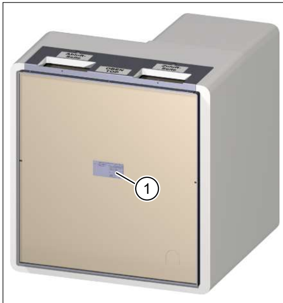
Fig. 2: Nameplate on the plaster cover
